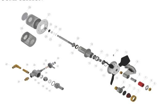
Image 01: Components of the Zanoni Equipamentos rotary atomizer®
