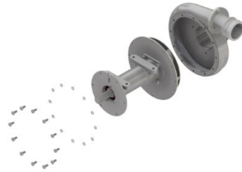
Figure 10: removal of screws from the seal cup assy.
