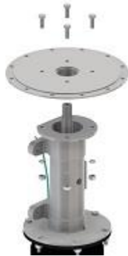
Figure 28: attaching the seal cup assy to the bearing housing.
