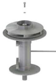
Figure 11: removal of the screws that put the impeller housing and the bearing housing together.
