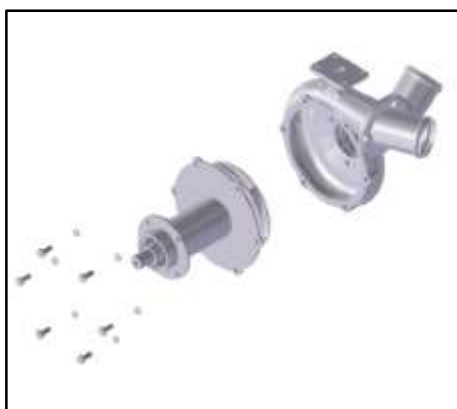
Figure 14: removing the screws that attach the impeller housing to the bearing housing.
