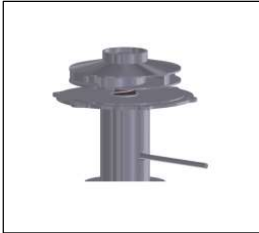
Figure 27: shaft locking to thread the impeller.
