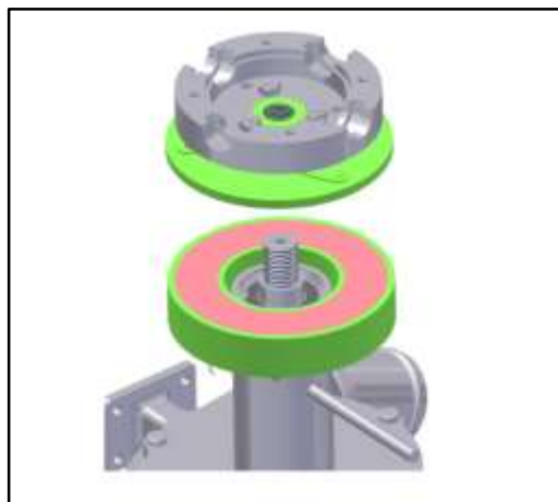
Figure 10: unscrewed brake assembly.
