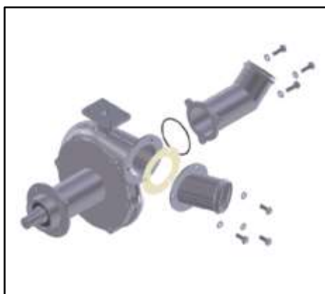
Figure 13: screws removed for replacing only the O'Ring or gaskets.
