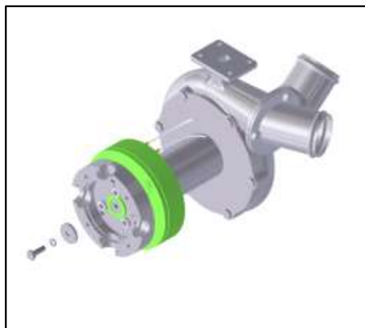
Figure 08: removing the safety washer.
