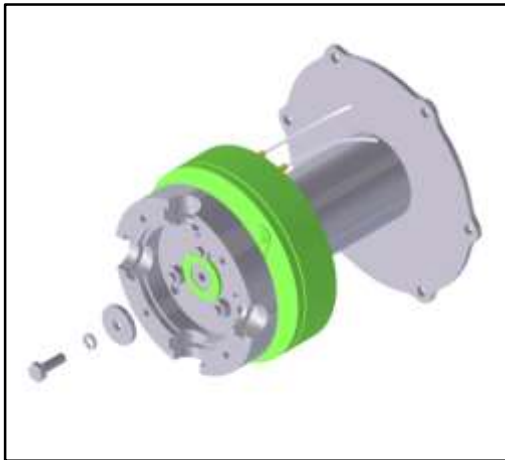
Figure 23: safety washer to ensure locking of the brake assembly.
